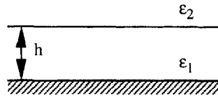
Fig. 7. Geometry of a microstrip substrate.
